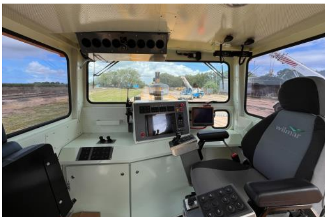
An internal view of the driver's cabin of the new Alma locomotive that has been introduced to Inkerman Mill
